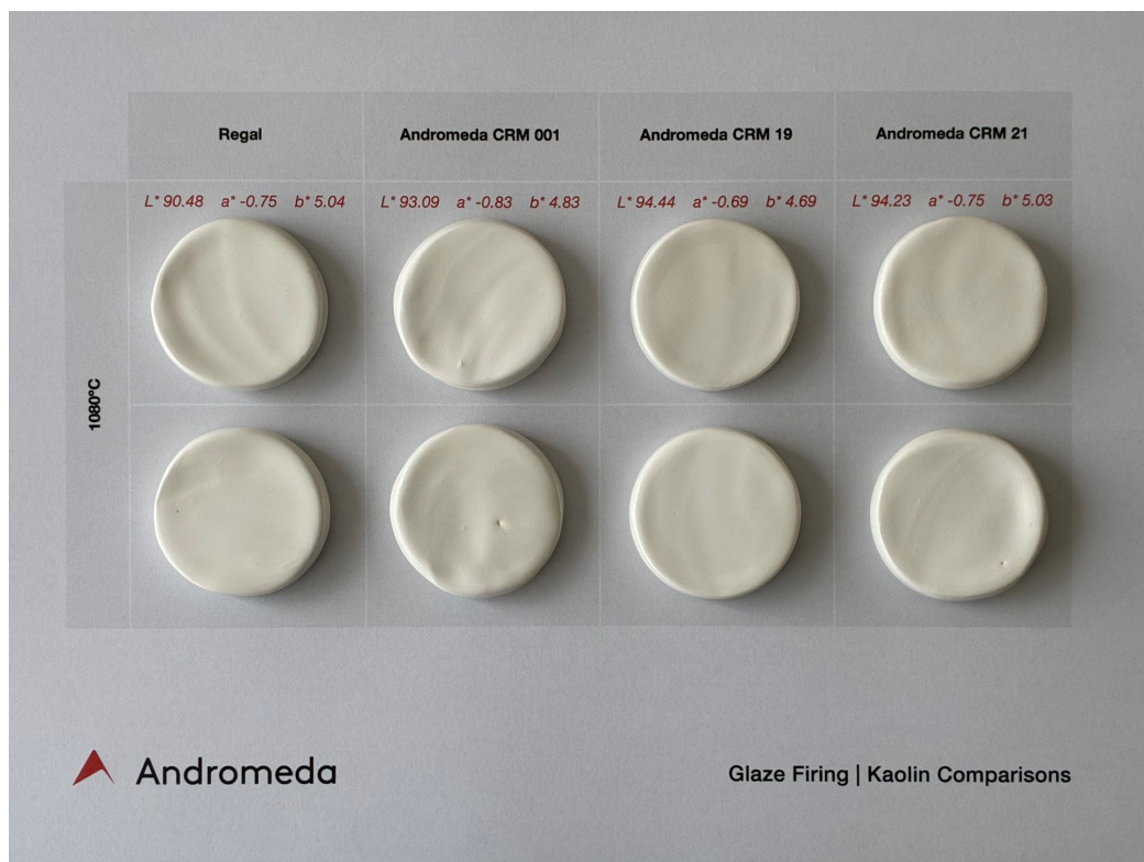
Figure 1 - Glazed discs after firing at 1080°C - UK standard glaze - (l to r) Chairlift CRM (CRM 001), Great White CRM™ P (CRM 19) and Great White CRM™ X (CRM 21)
