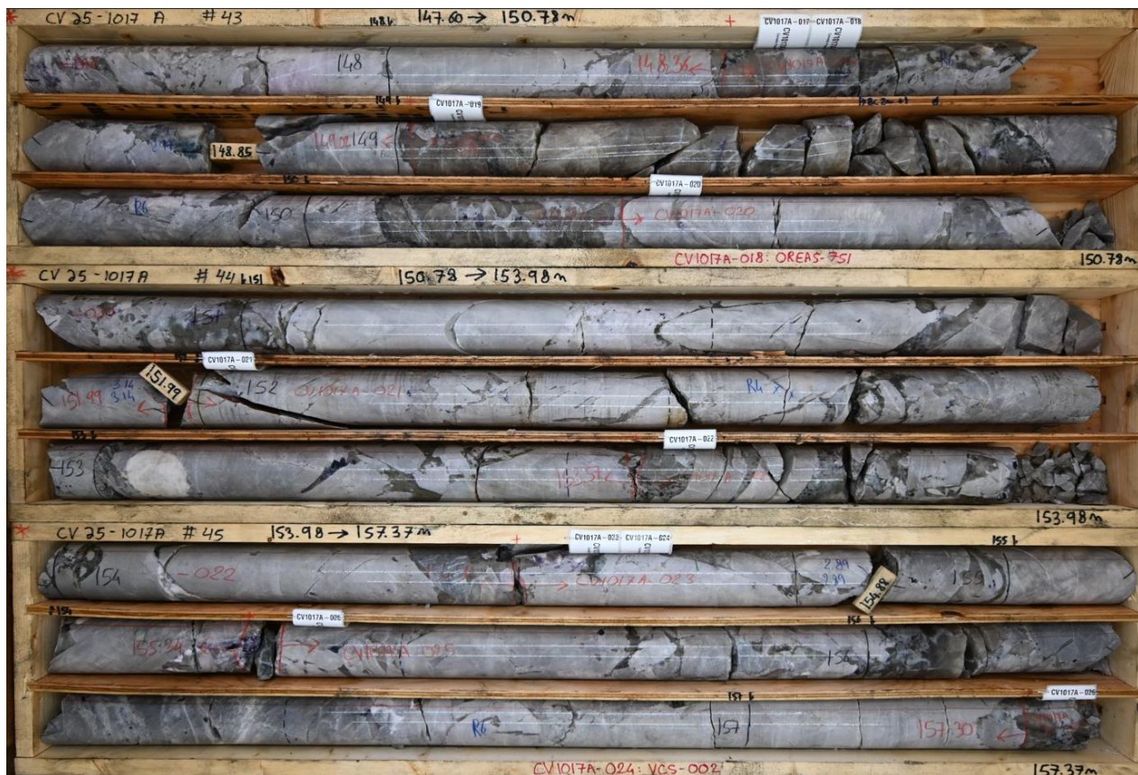
Figure 5: Abundant, large, and near-inclusion free spodumene crystals in drill hole CV25-1017A from the Vega Zone at the CV13 Pegmatite. Core grades 7.0 m at 6.04% \text{Li}_2\text{O} (from 150.3 m to 157.3 m) within a wider mineralized interval of 24.7 m at 4.00% \text{Li}_2\text{O} (146.0 m to 170.7 m).
