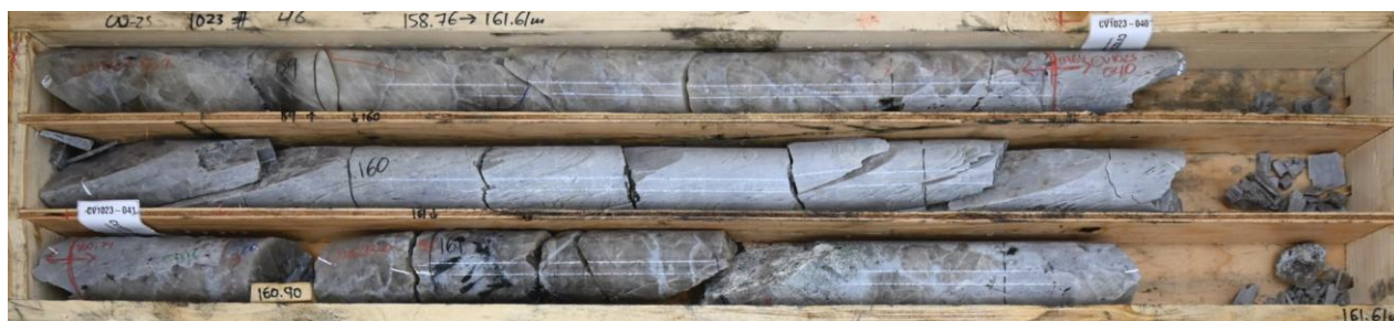
Figure 4: Massive and near-inclusion free spodumene in drill hole CV25-1023 from the Vega Zone at the CV13 Pegmatite. Core grades 1.1 m at 7.32% \text{Li}_2\text{O} (from 159.6 m to 160.7 m) within a wider mineralized interval of 31.2 m at 2.07% \text{Li}_2\text{O} (133.4 m to 164.6 m). At 7.32% \text{Li}_2\text{O} , this is the second highest grade of lithium returned from an individual core sample collected to date at the Property.
