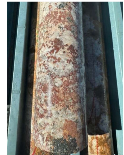
Image right: Visible rare earth mineral grains (red) in grey dolomite at 70m below surface
