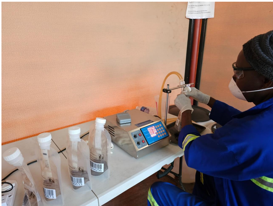
Figure 1: Sample preparation work underway at the at the PortablePPB laboratory established within the Dokwe Site Camp. These samples, once prepared, are then subjected to analysis via the DetectORE™ method using a pXRF device, which provides gold analytical data within 24 hours on site.
