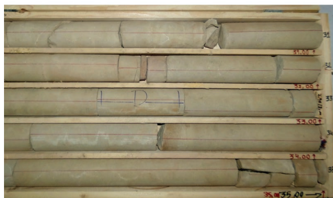
Figure 1 Diamond drill-core from hole GADD-05 – 30m depth to 35m.
