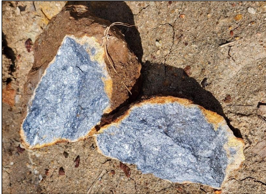
Figure 4: Massive Stibnite from sample BSE04 returning 55.5% Sb
