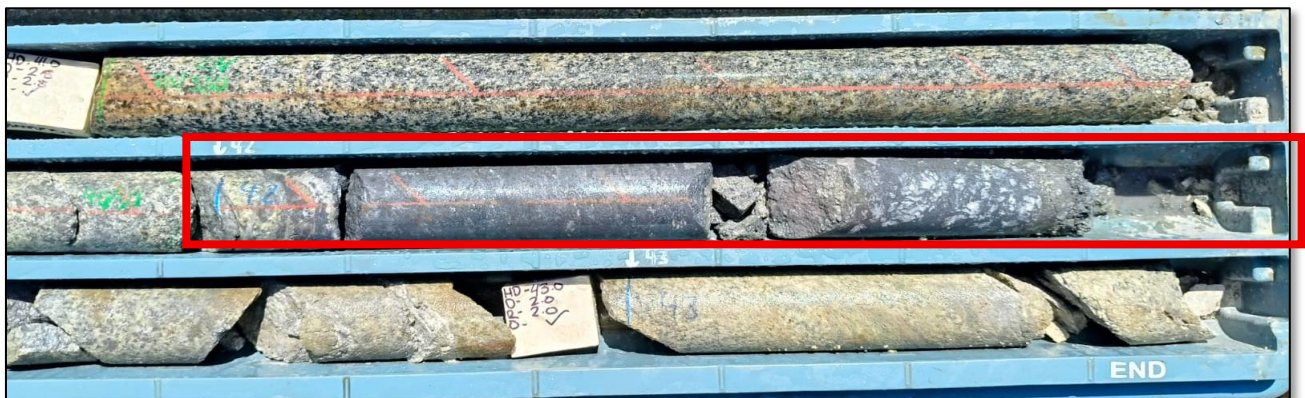
Figure 7: High-grade stibnite from Drill Hole CBADD001 showing massive sulphide, highlighted in Red, from 42m downhole. Estimation* of sulphide content is approximately 70% Stibnite, with assays expected to be returned in Early November.
