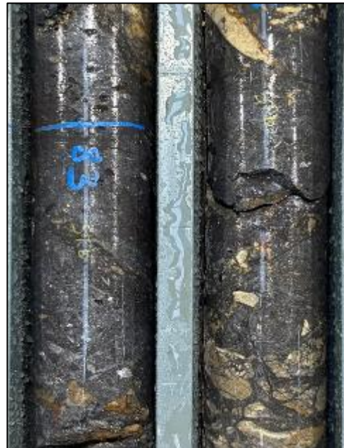
Photo 4. 19.61% Sb over 2.4m from 82m within 9.92% Sb over 4.8m from 81.5m (MAG010)
