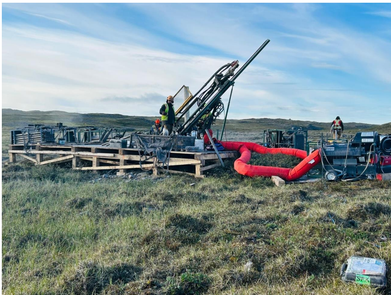
Figure 2 - Reverse circulation drilling underway at DAN25019
