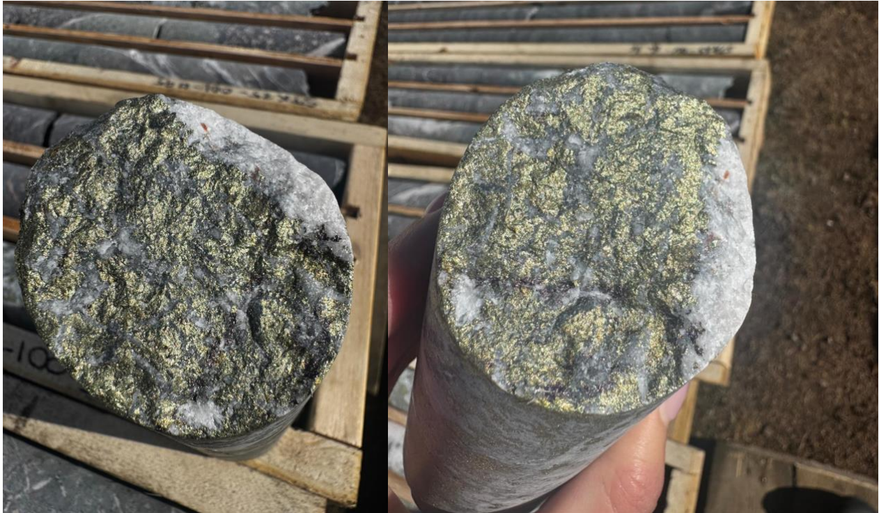
Figure 4 - Chalcopyrite-bornite-quartz-carbonate veining below the base of the sedimentary structure in STK25001 at 291.4m that returned assays of 14.95% Cu & 0.51g/t Au . Core diameter is NQ2.
