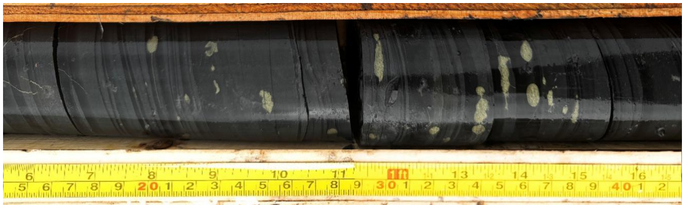
Figure 5 - Example of chalcopyrite replacement of inferred diagenetic pyrite nodules within reducing sediments of the lower Rae Group between 182.24 and 182.52m downhole in STK25001 that returned assays of 1.2% Cu . Core diameter is NQ2.
