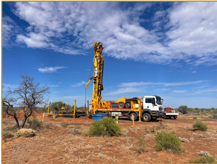
Figure 4. Core drilling at the Byro Project.
