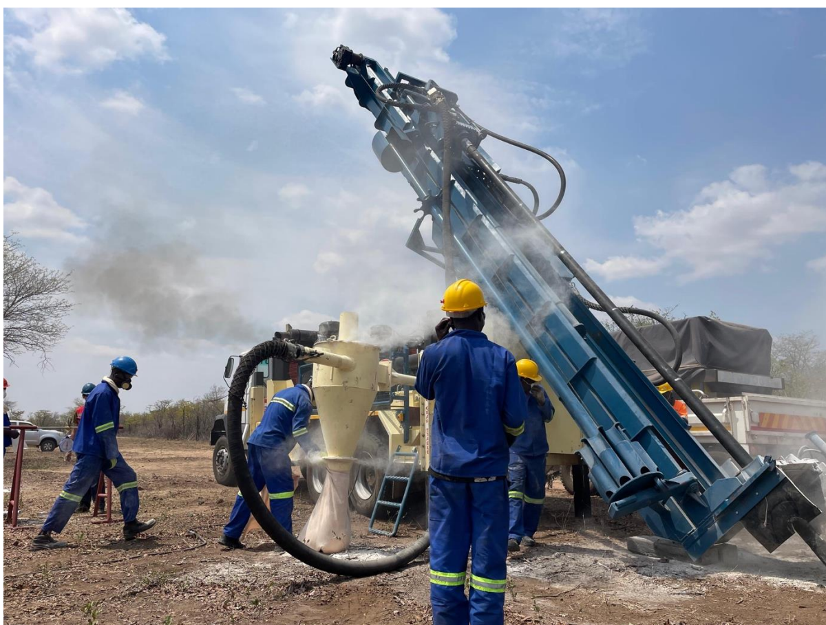
Figure 1: RC drilling commences at the Dokwe Project. Several targets are being tested, including the gold-in-soil anomaly identified to the northeast of Dokwe North and various targets in the vicinity of Dokwe Central.
