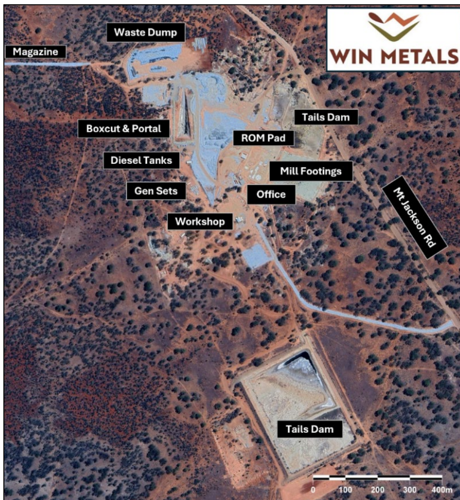
Figure 8: Radio Mine Site Layout and Infrastructure
