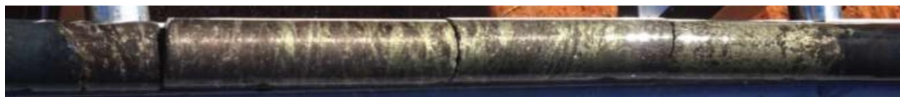
Figure 3. 60 cm long section of unweathered massive sulphide from PSD02 with textures typical of magmatic nickel-copper sulphides.
