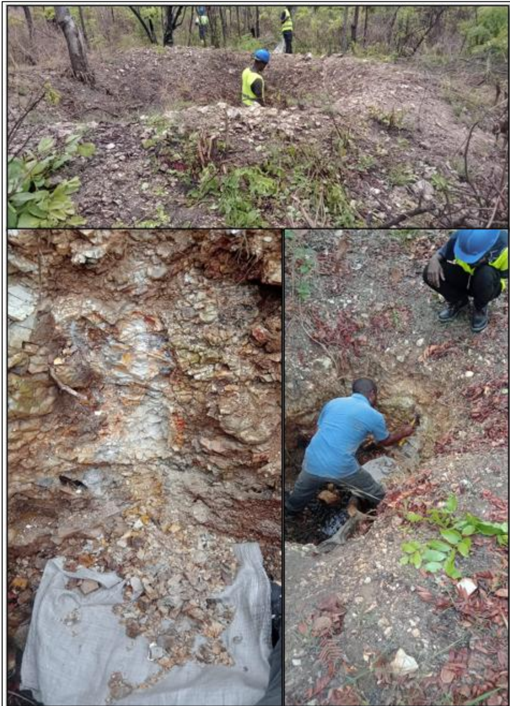
Figure 1: Artisanal test pits found within Adriano 11002 in pegmatite rocks. Images show the sampling taking place of the pegmatites.
