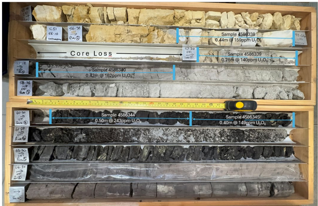
Figure 2: Core hole C51, with significant uranium assay intersections marked. Note redox boundary becoming evident in the sample 4586338 sample interval.
