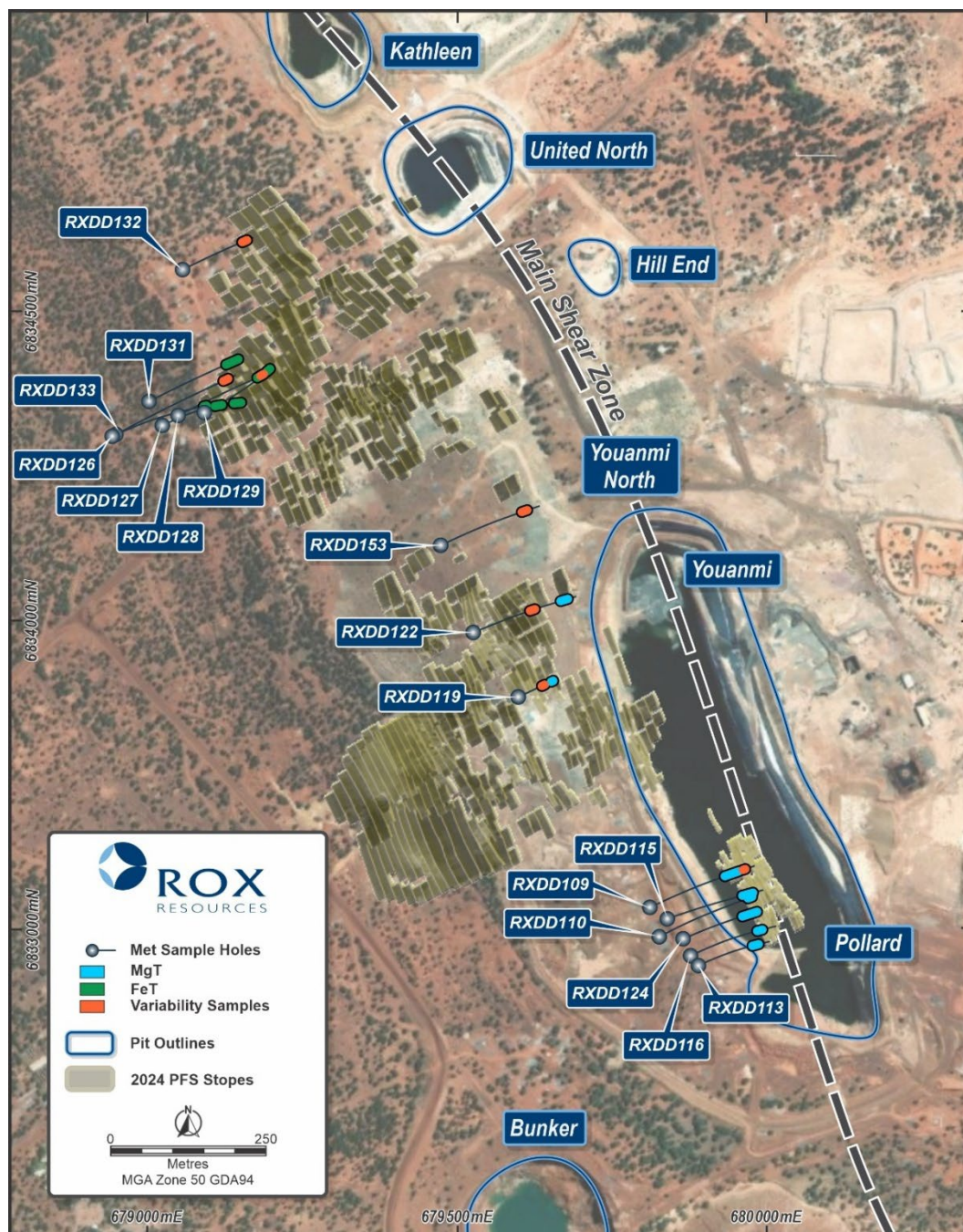
Figure 20. Metallurgical Composite Sample Selection Locations
