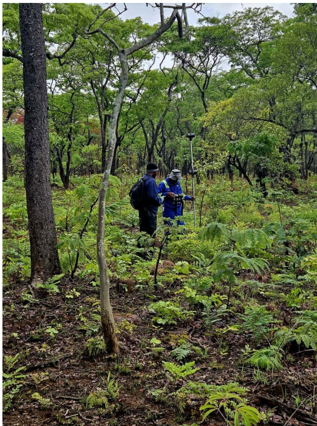
Figure 3: Ground magnetics survey in progress, with I.P. to follow at Target B1
