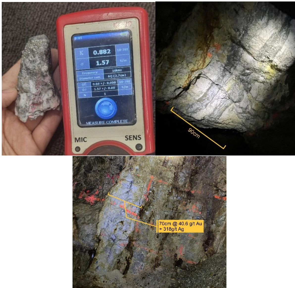
Figure 2: (left) Very high grade grab sample (358.0g/t Au & 1,800g/t Ag) showing typical magnetic susceptibility & conductivity readings. Figure 3: (right) Banded sulphides in the backs of the South Black Bear Vein. Figure 4: (bottom) Western face of the South Black Bear Drive (0.7m @ 40.7g/t Au & 318g/t Ag)
