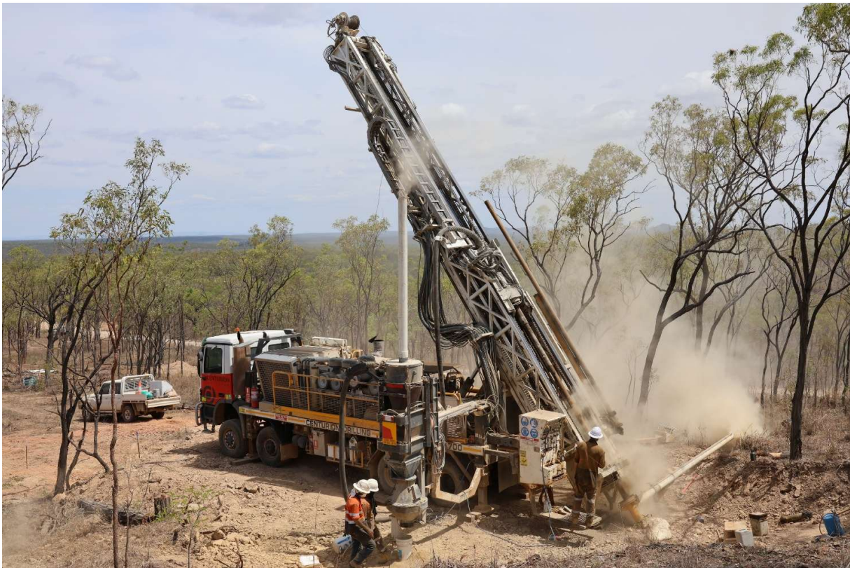
Photo 1: RC Drilling rig in operation at St George Gold-Antimony Project in northeast Queensland.
