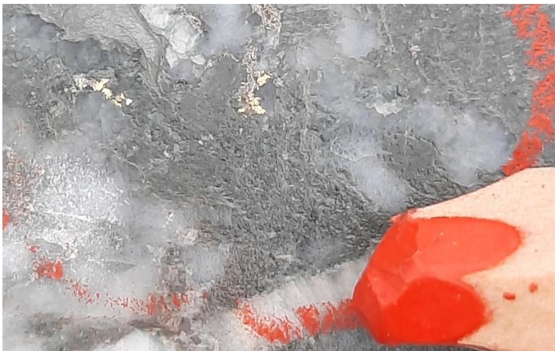
Figure 4. Multiple patches of visible gold up to 2.5mm (lustrous yellow) within an irregular quartz stockwork zone in hole AMD014A at 466.0m. Assays are currently pending for this hole. Note: In relation to the disclosure of visible mineralisation, the Company cautions that visual estimates of mineral abundance should never be considered a proxy or substitute for laboratory analysis. Laboratory assay results are required to determine actual widths and grade of the visible mineralisation reported in preliminary geological logging.
