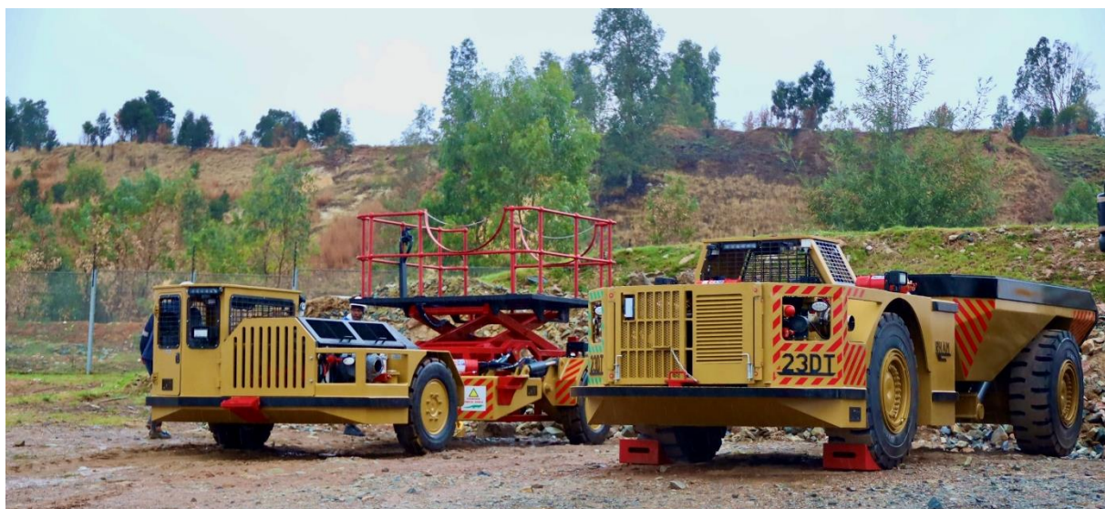
IMAGE 3: DUMP TRUCK COMMISSIONED AND MULTI-PURPOSE UTILITY VEHICLE FOR MATERIAL TRANSPORT AND UNDERGROUND INSTALLATIONS
