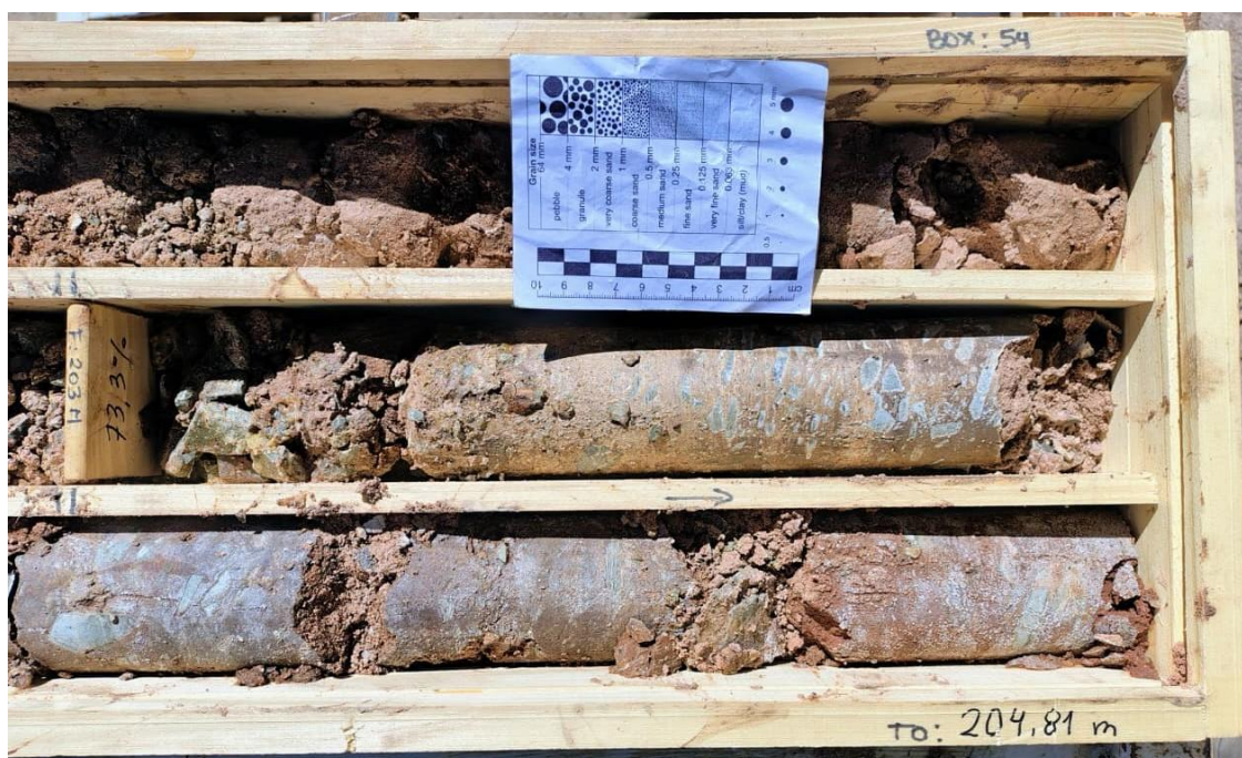
Figure 5. Core from (199.9 - 206 m): Unconsolidated, light brown medium to coarse gravel with medium to coarse sand matrix, matrix-supported, with sub-angular clasts. Moderate-high porosity.
