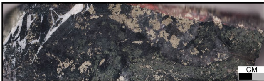
SPD015 295.5 m (Consols, HQ Core). Albite-hematite altered andesitic psuedo-breccia with overprinting quartz-pyrite mineralisation and late carbonate crackle-breccia. 29.76 g/t Au.
