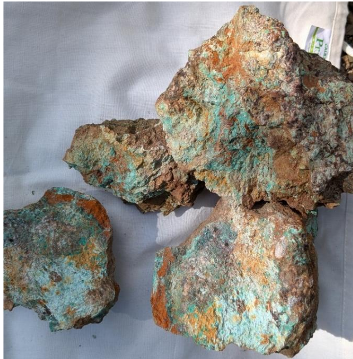
Figure 3: Rock chip sample RK010: 15.25% Cu
