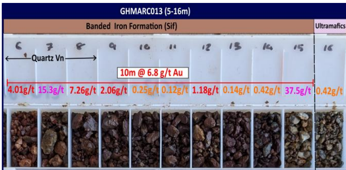
Figure 4: GHMARC013 RC chip tray showing 10m @ 6.8 g/t Au from 5m.
