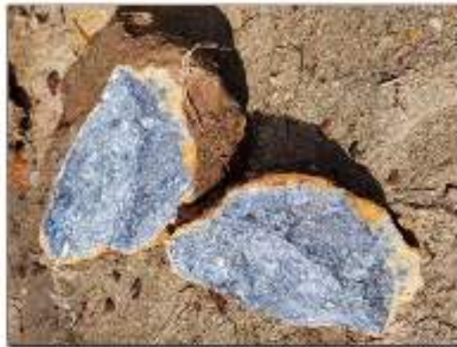
Figure 1: Massive Sb 2 S 3 from sample BSE04 returning 55.5% Sb
