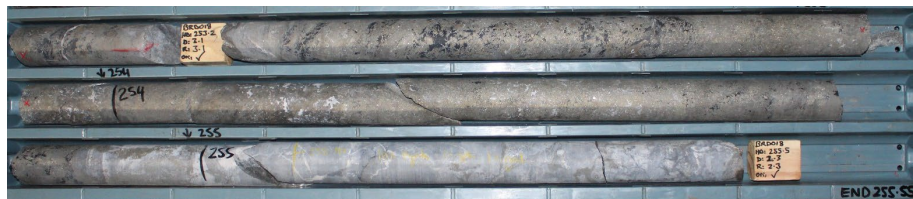
BRD018 , massive sulphide mineralisation (253.0-255.5m)
