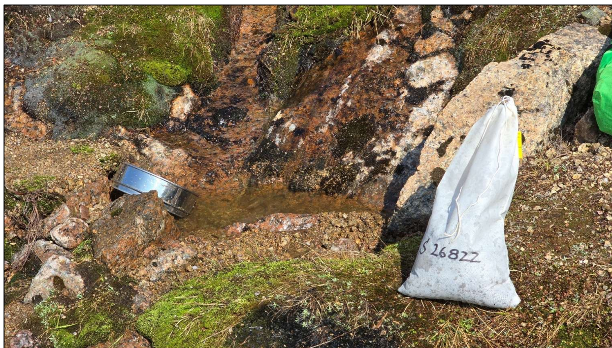
Figure 2: Field photograph showing sediment sampling at Blue Lagoon (Sample S26822). Photo illustrates coarse feldspathic sand and granitic fragments at a seepage zone near Blue Lagoon within the southern project area. Note the stainless-steel sieve used during field sampling and the tagged sample bag (S26822) ready for export.
