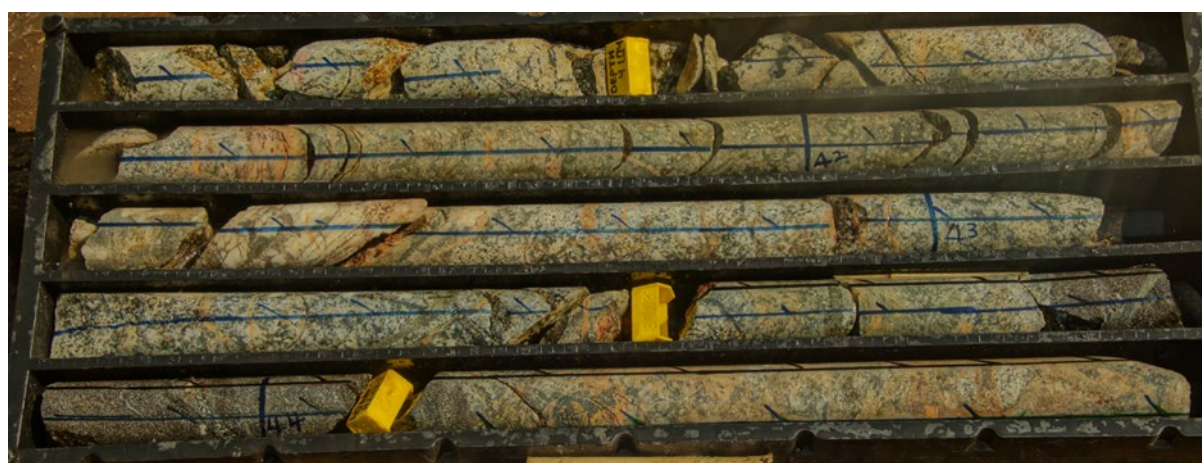
Figure 4. Diamond drill core from hole MDD 006 (metallurgical DD hole) containing potential REE mineralisation from visual inspection (pinkish coral colour) from approximately 41m to 45m down hole
