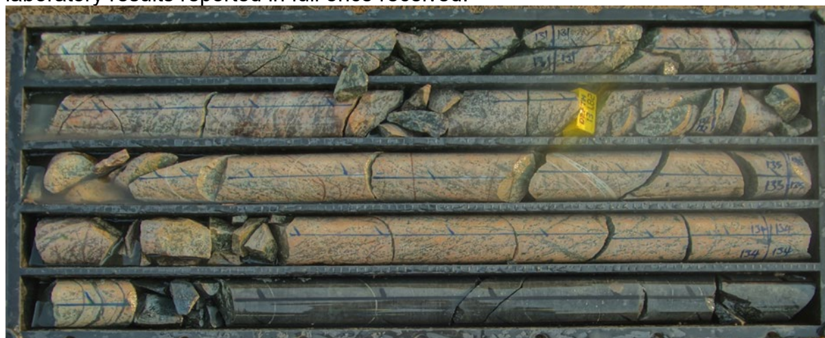
Figure 2. Diamond drill core from hole MDD 005 containing potential REE mineralisation from visual inspection (pinkish coral colour) from approximately 130m to 135m down hole
