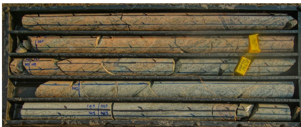
Figure 3. Diamond drill core from hole MDD 005 containing potential REE mineralisation from visual inspection (pinkish coral colour) from approximately 139m to 143m down hole
