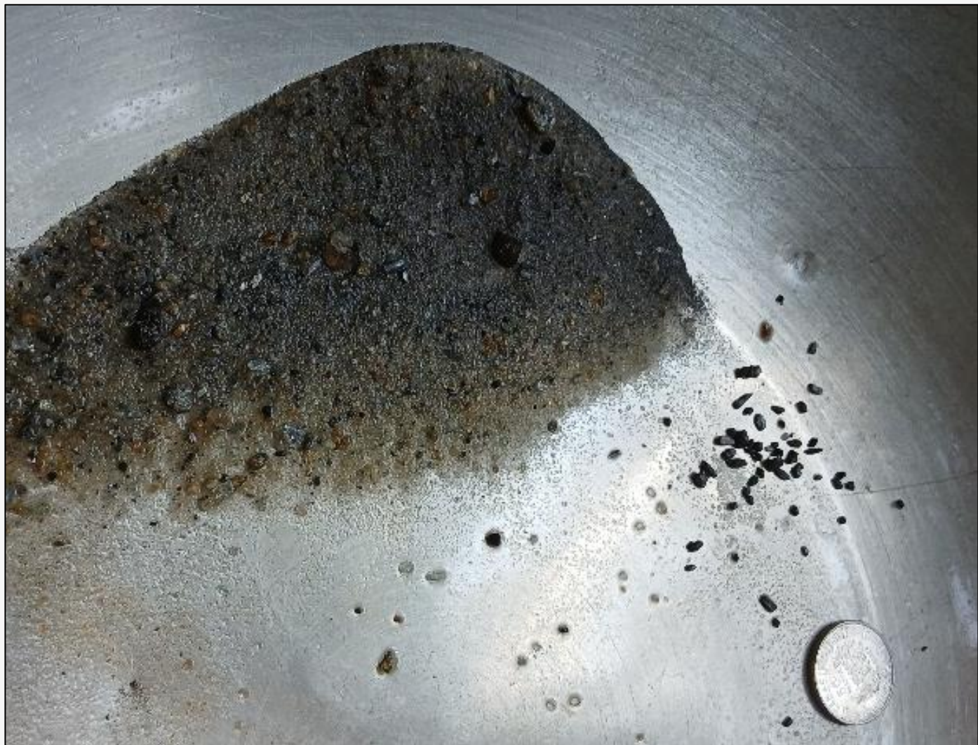
Figure: Fine-grained heavy mineral (HM) and rutile grains (~1 mm) recovered from a panned concentrate of auger hole GRMAU0004 (not assayed). For assay results from this hole, refer to ASX announcement: 2 September 2025 - High-grade saprolite-hosted rutile confirmed at Central Rutile Project (0.95 m @ 11.52% HM, including 0.96% rutile)
