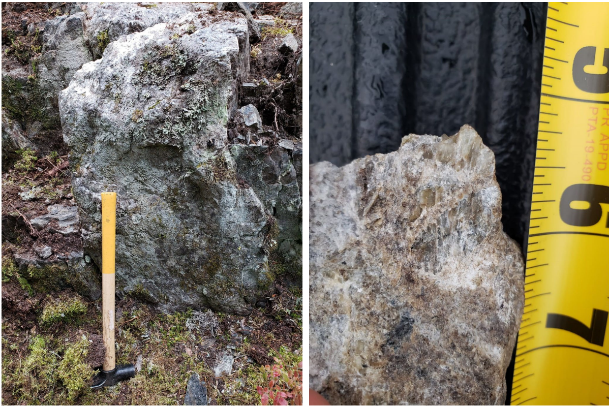
Figure 2. Photo of spodumene-bearing pegmatite outcrop hosted within metasediments (left) and medium-grained spodumene lathes within a pegmatite sample (right) from the Central Corridor 2 . Refer to Table 1 for further details.
