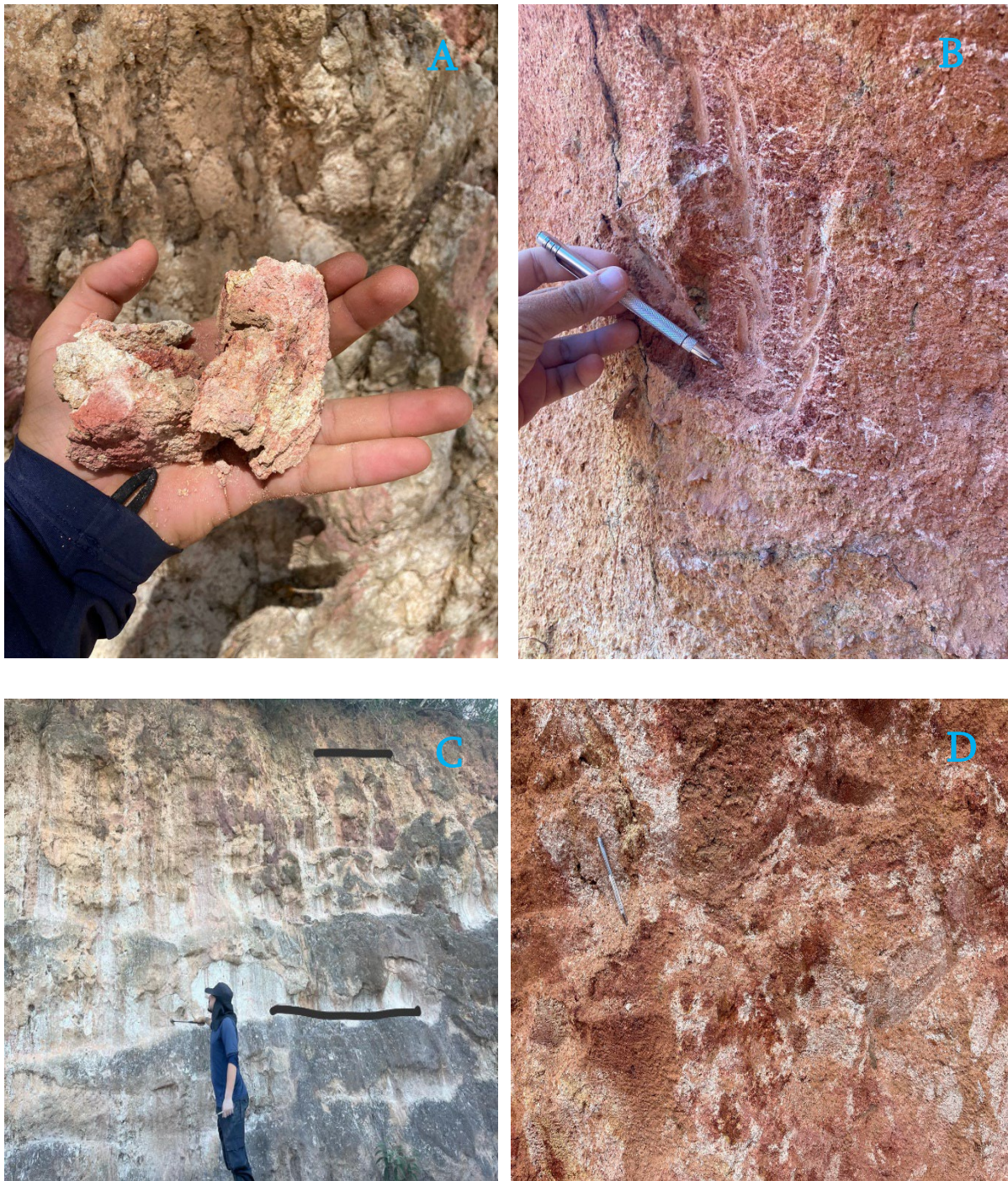
Figure 2- (A) Clay soil with beige and pinkish hues; (B) Silty soil with quartz fragments and clay minerals; (C) Outcrop approximately 5 meters tall with slightly weathered saprolite in the lower portion, more weathered clayey saprolite in the middle portion, and soil with organic matter in the upper portion; and (D) Residual saprolitic soil rich in clay minerals with a speckled texture from the Verde Valor tenements.
