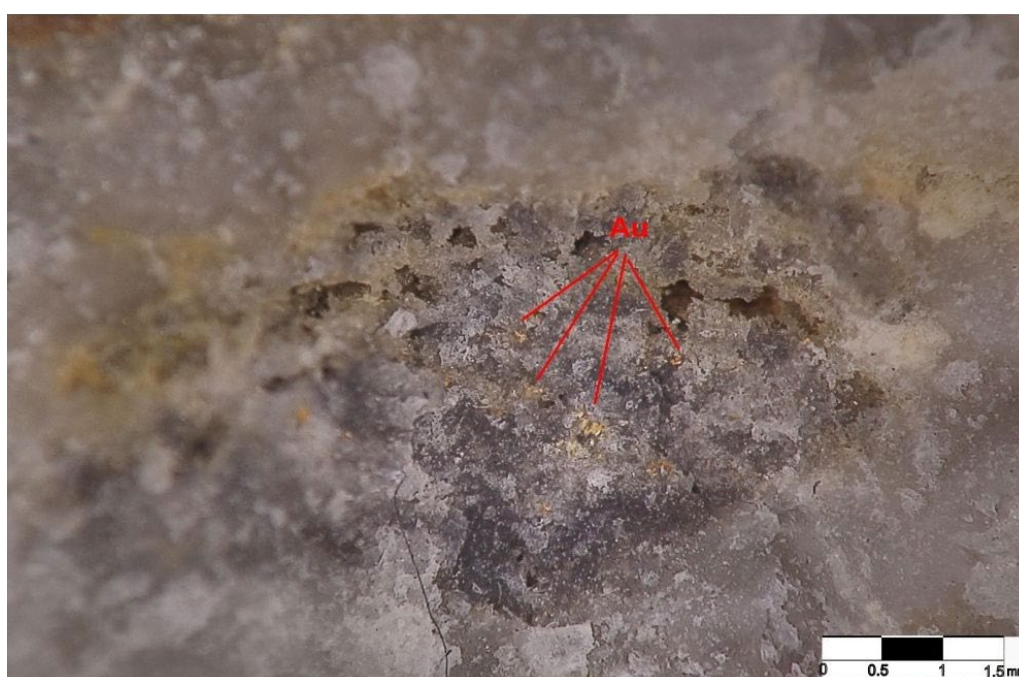
Fig. 1: Native gold aggregates in sample no. 387051 from Waitekauri. Native gold alloy consists of relative distribution (not total rock concentration) 68% Au and 32% Ag. Field of view is approx. 8mm.
