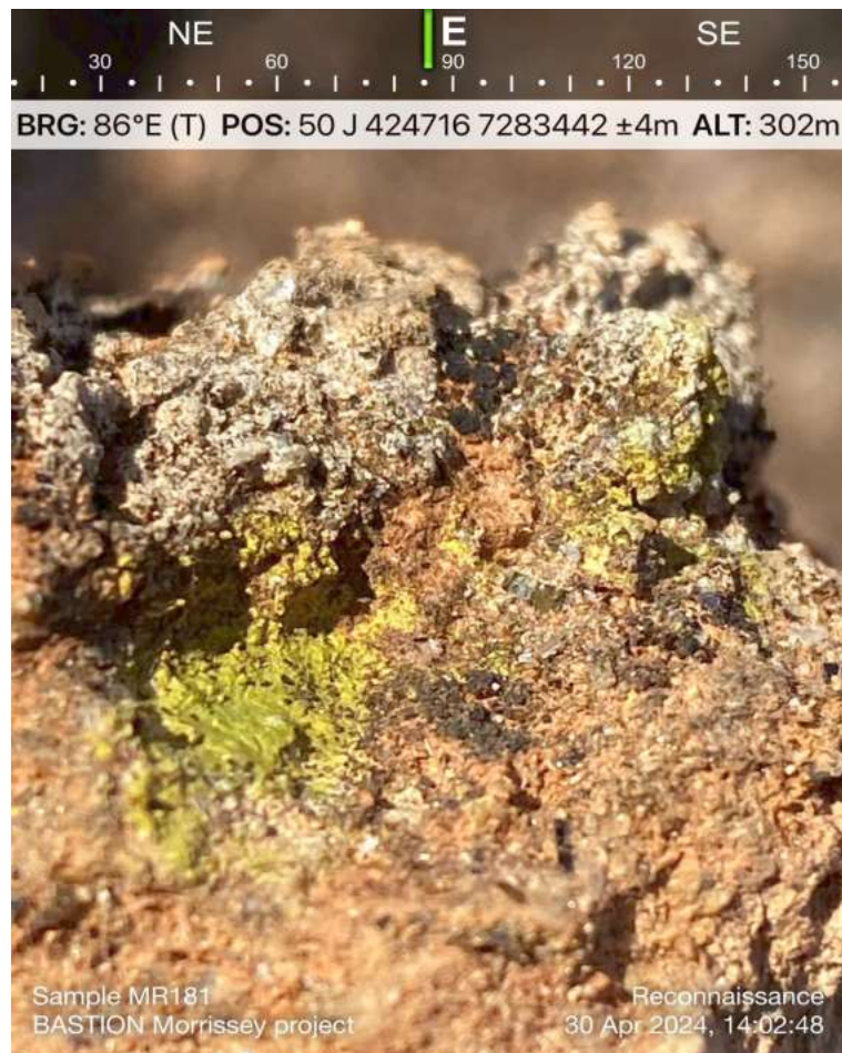
Figure 6: Visible disseminated and discordant Carnotite (Uranium oxide) mineralisation at sample MR181 site (424714E, 7283440N, UTM Zone 50) in the west of the property. ( \leq 1\% visual estimate of carnotite).
