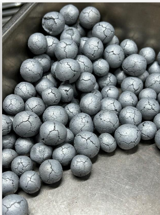
Picture 2. Pellets after Linder metallisation/reduction
