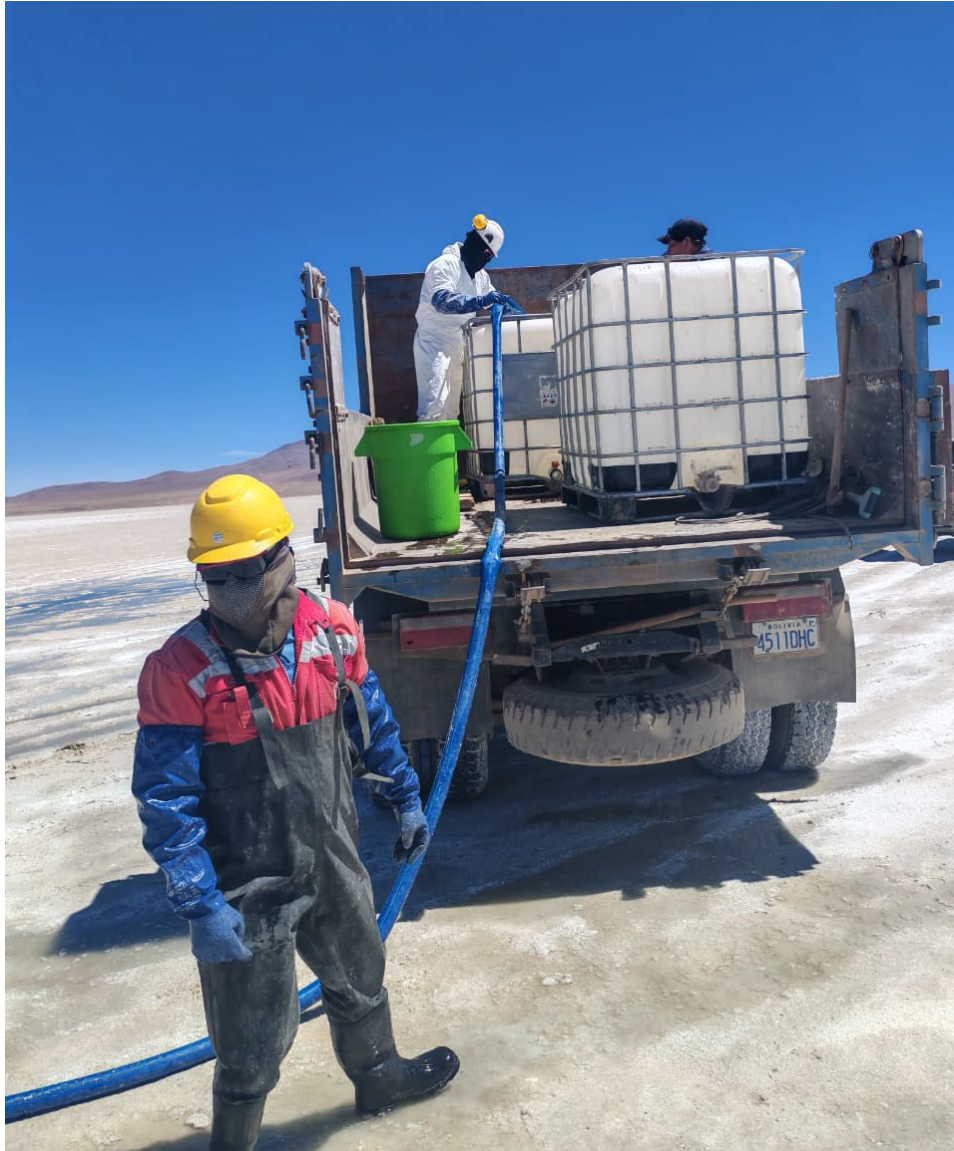
Figure 2 – Brine Transfer into Bulk Containers at Salar de Pastos Grandes for Transport and Testing
