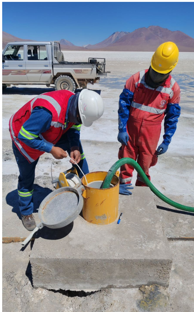
Figure 1 – Brine sample collection at Salar de Pastos Grandes for testing with Vulcan's proprietary VULSORB® technology. The process involved purging the well (above) before pumping brine into bulk containers (Figure 2). This procedure was also repeated at Salar de Coipasa and Salar de Empexa.
