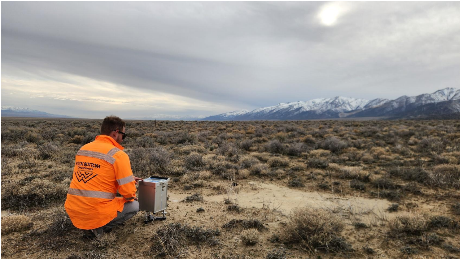
Figure 1; Photo showing collection of gravity data at the Linka Tungsten Project, Nevada, USA
