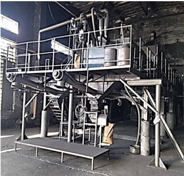
Figure 1: Zavalievsky Graphite purification circuit used to produce 99.5% high purity graphite in Ukraine.
