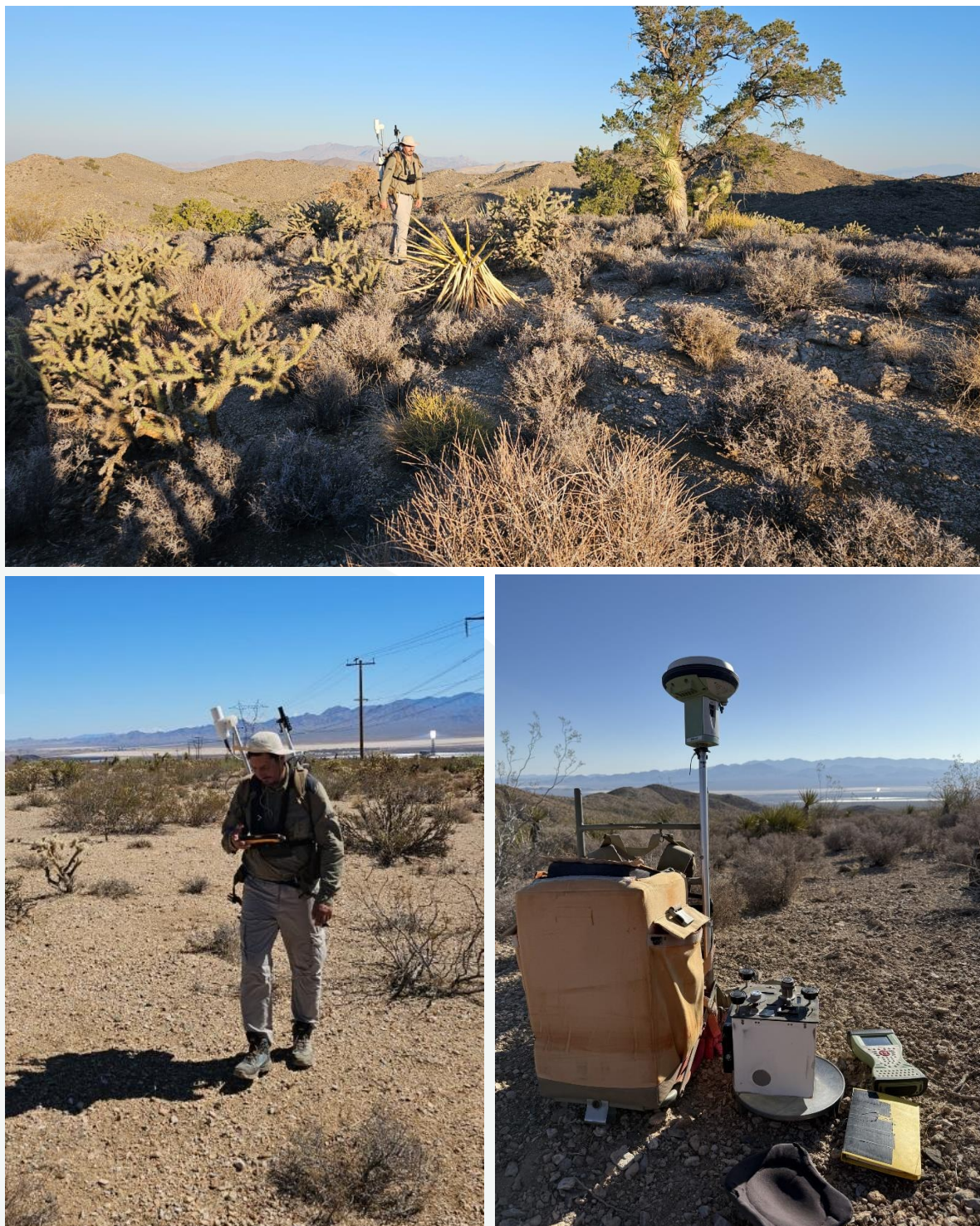
Figure 4: Field crew conducting ground magnetic and gravity survey at Desert Star Project
