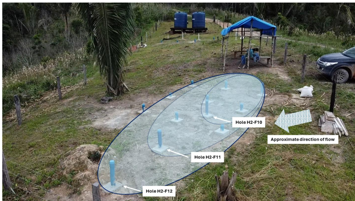
Figure 2. Field pilot trial and setup showing distribution of monitoring holes H2-F10, H2-F11, H2-F12. Rings indicate approximate area of leaching influencing grades received from the PLS, with H2-F10 being the smallest leaching area.
