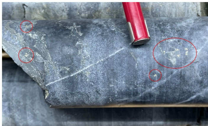
Figure 2 (RHS): Visible gold grains in 20cm smoky quartz vein hosted in sulphide, chlorite-carbonate altered wacke, 187.85-187.90m, BO-25-27. Core diameter is 4.76 cm.
