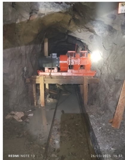
Underground mine scrapers introduced to assist in ore delivery from the stopes, Santa Barbara gold project
