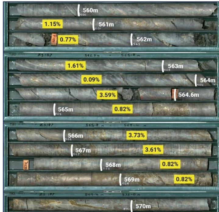
Photo 1: Drill core from ZS187, 560 – 570.5m down hole showing upper lode intersection of 10.2m @ 1.68% Sn from 560m, including 4.0m @ 2.94% Sn from 564m.
