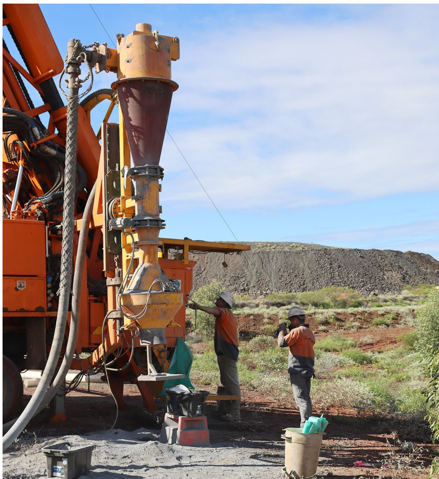
Photo 1. Running in the Gyro for a downhole survey (GAM drill program).
