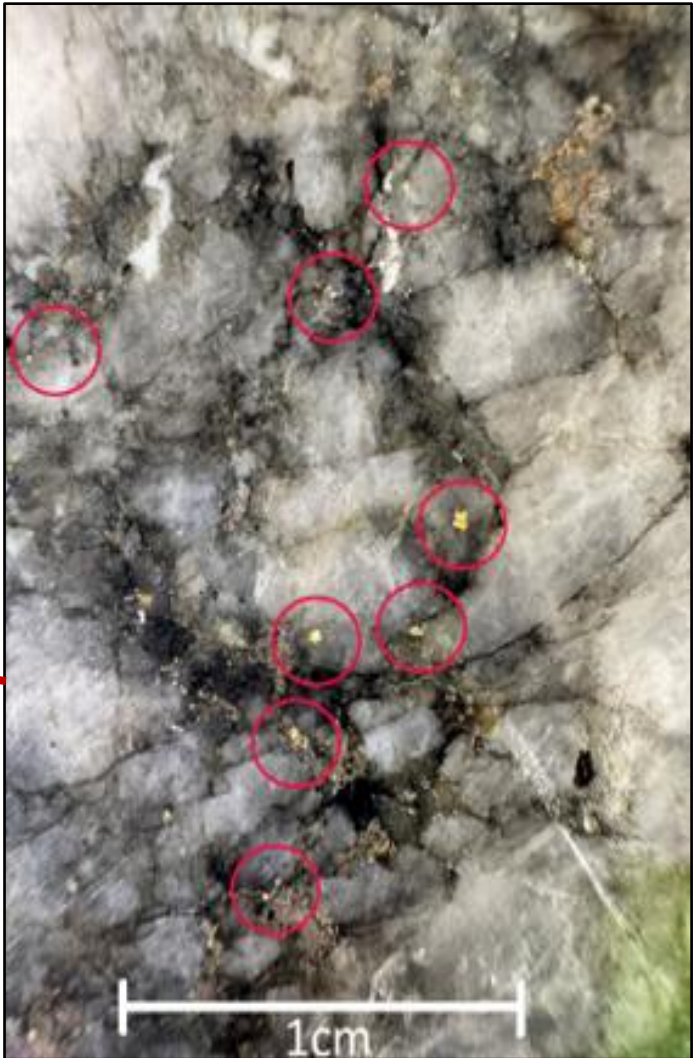
Drill core with visible gold (0.2m @ 629g/t Au from 244.1m) from hole BBDD0021
