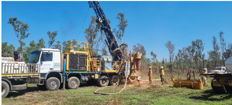
Aircore drilling in the field at EverGreen's EL 31774
