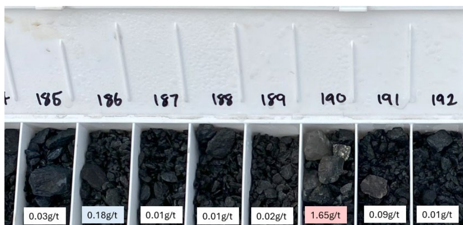
Figure 3: SMX001 (Reverse circulation hole) – quartz, sulphide returned assay grade of 1m@ 1.65g/t from 189-190m 4 . Assay results of each metre shown.
