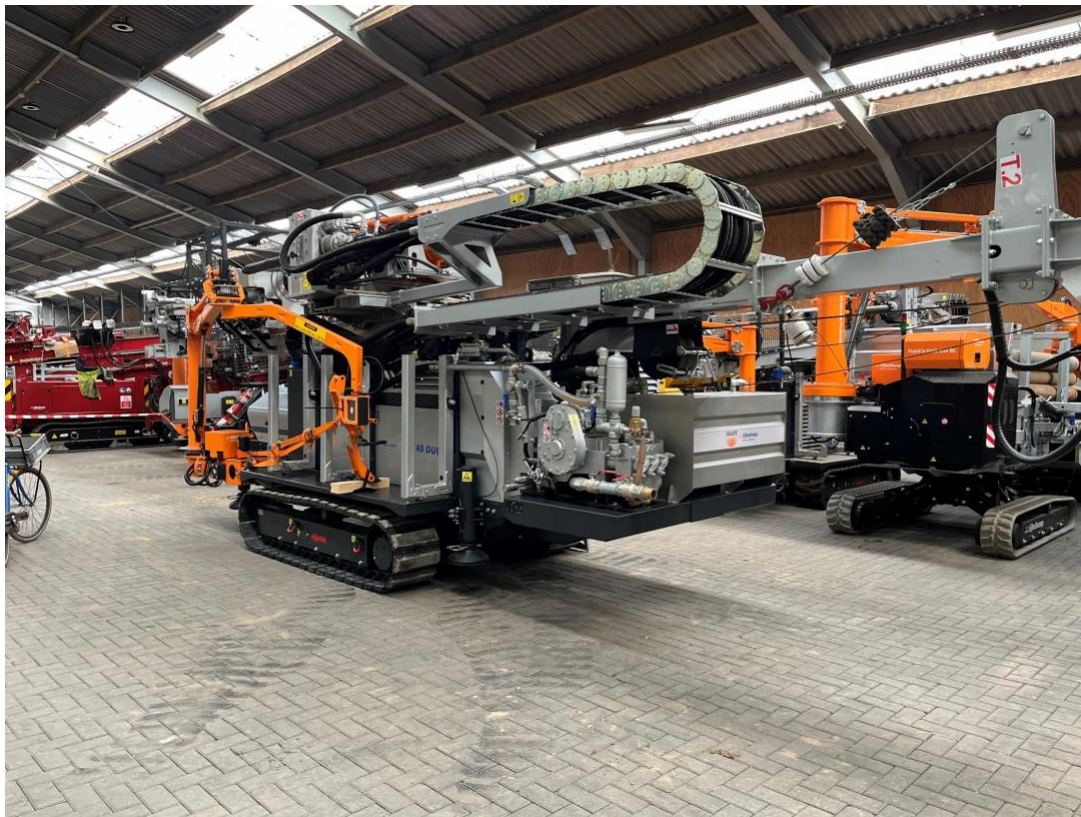
Figure 1: Photo of the new sonic drill rig to be deployed to site in November
