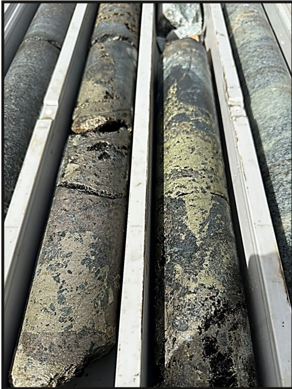
Figure 3 – Massive sulphide mineralisation within hole 24NRDD0125 contained within interval 234.1-236.2m.
