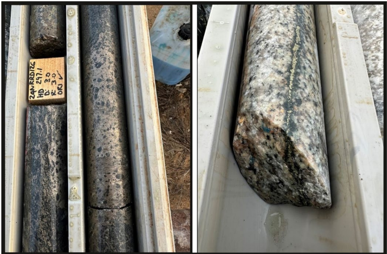
Figure 2 – Massive (left) and veined (right) sulphide mineralisation within hole 24NRDD0126 contained within interval 295.1 -300.3m (5.2m).
