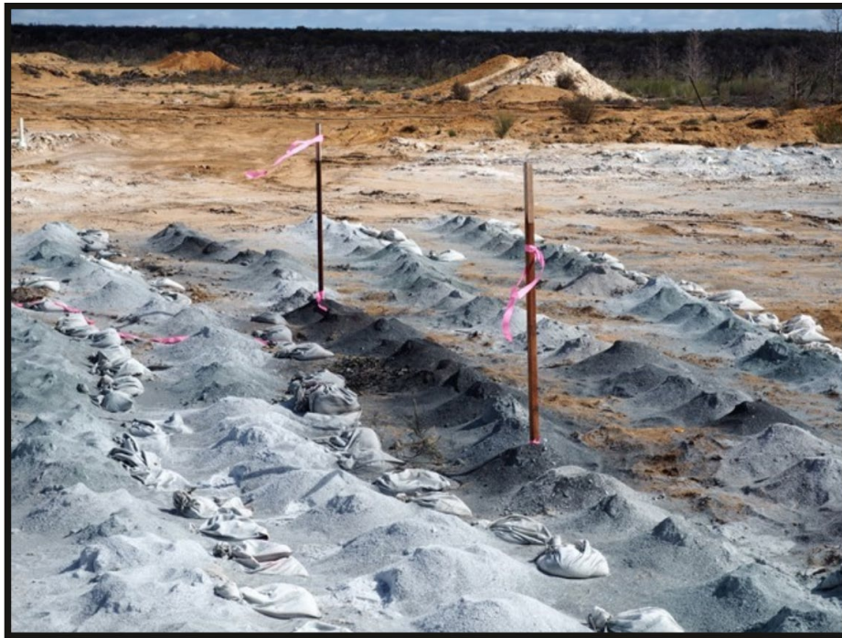
Figure 1 – 24NRRC0124 R/C Drill piles, black material represents massive sulphide intersections (128-138m marked by wooden pegs).
