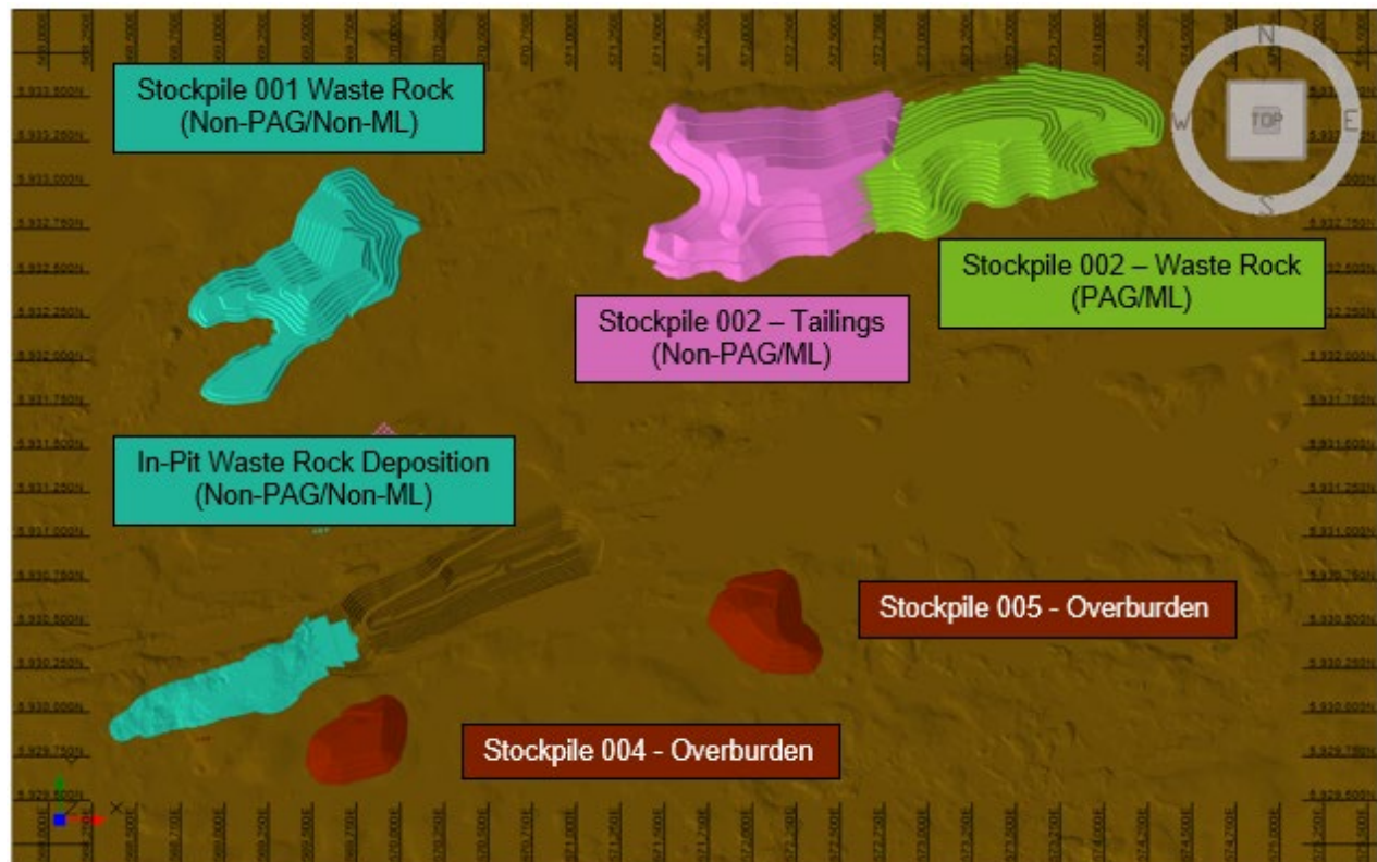
Figure 10: Overburden, Waste Rock and Tailings Storage Facilities – Plan View (Not to scale).
