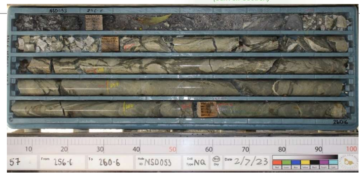
NSD053 – weakly sericitized basalt beneath mineralisation
