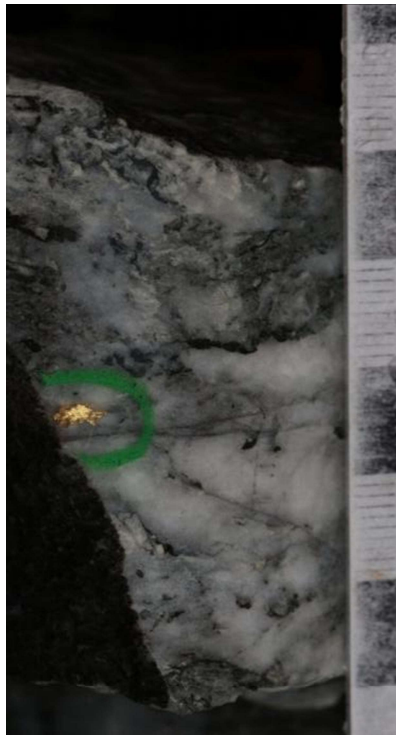
NSD057 – 108.2-109m includes multiple instances of visible gold (VG) in quartz veining. This is not a typical mineralisation-style for NSM –the geology, mineralisation and structure have strong similarities to the historic Mariners mines that boasted an historic production grade of ~30 g/t Au.
